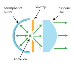
The ability to observe the spontaneous emission behavior of atoms can aid in the study of many quantum electrodynamics (QED) phenomena. Looking for a way to measure these emissions, Araneda et al. designed a unique mirror-integrated ion trapping system, which they named "Panopticon."
