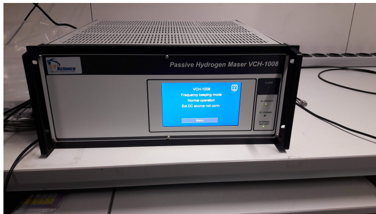
Figure 4.12: Photography of passive hydrogen maser VCH-1008.
