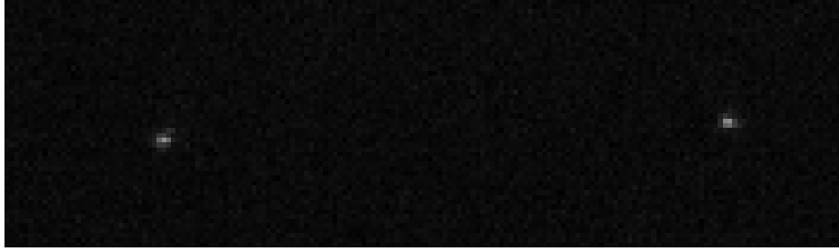
Figure 3.14.: Overlay of two camera pictures with 100 MHz (left spot) and 60 MHz (right spot) applied to the AOD. The distance between the two spots is 119 pixels, corresponding to 199 \mu\text{m} .
