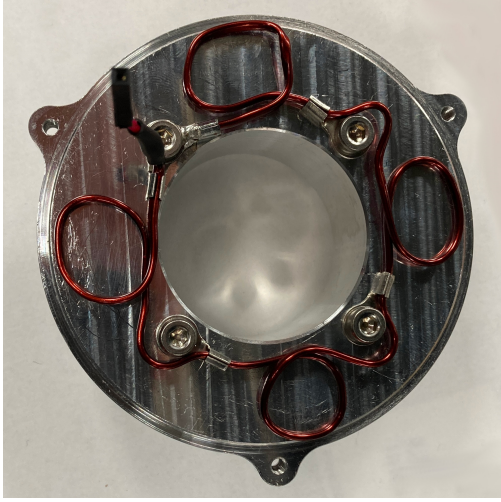
Figure 4.3.: Image of the pickoff coil, screwed onto the baseplate, before mounting it together with the resonator on top of the vacuum chamber. While the pickoff coil was newly built, the baseplate is part of the existing helical resonator design from [116]. On the top left, one can see the pin connector which, when mounted, is plugged to the SMA connector on the inside of the resonator's shield (see (9) in Figure 4.2).
