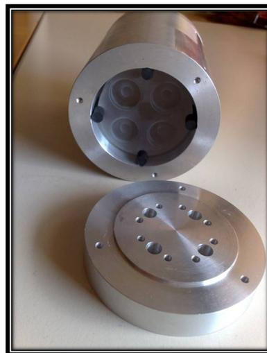
(b) Front view of the cavity with vacuum housing
